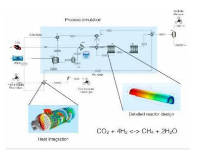
Figure 2 – Synthesis of Methane and Heat Recovery (SOMAHR)
